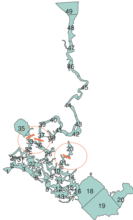
Figure 26. Recommended Segments for building artificial waterfalls
