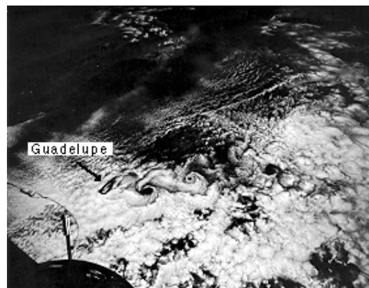
Figure 38 - Examples of vortex streets behind an island observed in the atmosphere. The island of Guadelupe is seen to produce a von Karman vortex street. Two vortices are visible in the first image, the vortices on the other side of the vortex street cannot be seen because of a break in the cloud cover; the image is adapted from NASA (1968).
