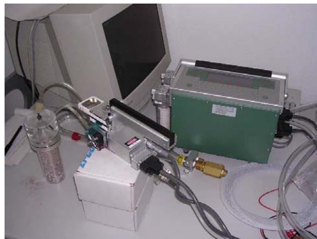
(Measuring sediment respiration under different hydrologic conditions using a LICOR-gas chromatograph (EAWAG))
