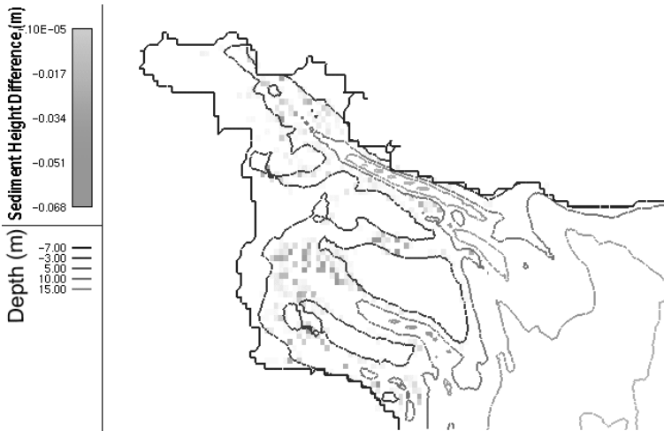
FIGURE 14: Sediment height difference between the last three years simulated with an erosion rate of 10^{-5} \text{ kg m}^{-2} \text{ s}^{-1} .
