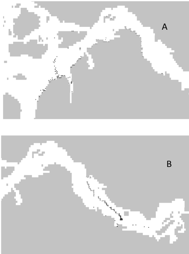
FIGURE 3: Spatial distribution of lagrangian drifters for the first experiment, non-sinking drifters (A) and the second experiment (sinking drifters) after 36 hours of simulation.
