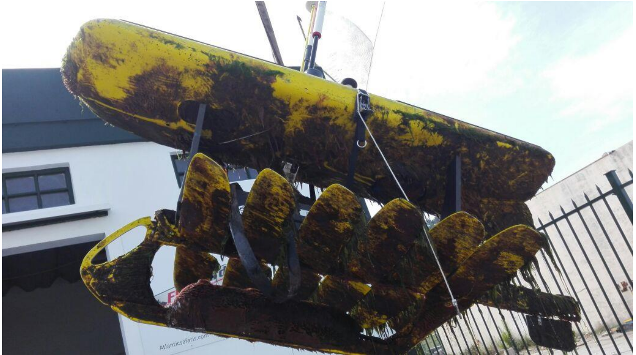
Picture 3 The WaveGlider SV2 Hermes after its final recovery with covered with fouling organism. (Credits: Atlantic Safaris).
