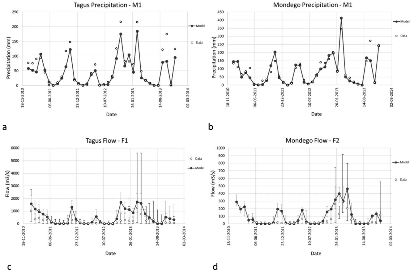
**Fig. 3.** Monthly averaged modelling results (solid line) and observations (white circles) for the Tagus River (left side) and for the Mondego River (right side) for precipitation (top) and river flow (bottom) for the period 2011–2013. The graphs include error bars for flow observations (black bars) and for the flow modelling results (grey bars). Error bars for model precipitation are not visible, as the standard deviation values are too small.
