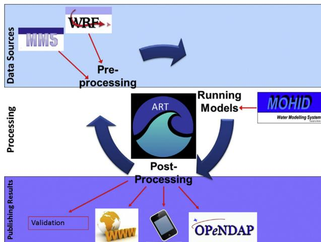
Fig. 2. General scheme of the Automatic Running Tool (ART) where it can be distinguished the pre-processing, modelling and post-processing cycle of operations including only elements used for the WI and IP Mohid Land applications.
