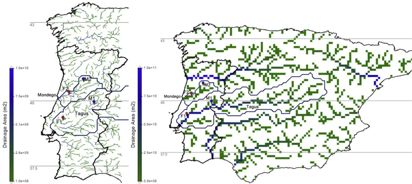
**Fig. 1.** Main water lines in the Western Iberian Peninsula (WI domain, left) and in the complete Iberian Peninsula (IP domain, right) indicating the drainage area obtained with the MOHID Land for the 2 and 10 km resolutions respectively and the location of the hydrological (F1 and F2) and meteorological (M1 and M2) stations used for the model validation. The drained area by the Mondego River and the Tagus River appears enclosed by continuous lines in both domains.
