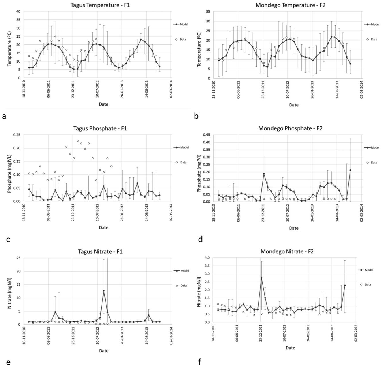
**Fig. 6.** Monthly averaged modelling results on river water quality (grey line) and station field data (white circles) for the Tagus River (left) and Mondego River (Right); a) and b) temperature (°C); c) and d) orthophosphate ( $\text{mg P l}^{-1}$ ); e) and f) nitrate ( $\text{mg N l}^{-1}$ ). Error bars are only shown for modelling results as the observed values correspond to monthly samples.
